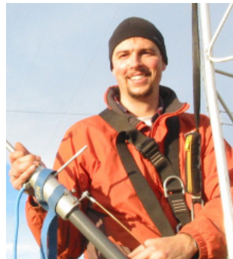
Chris Thomas installing a sonic anemometer that measures high-resolution wind speed and temperature to quantify air-vegetation interaction. Photo by bMM group, http://oregonstate.edu/bmm/
