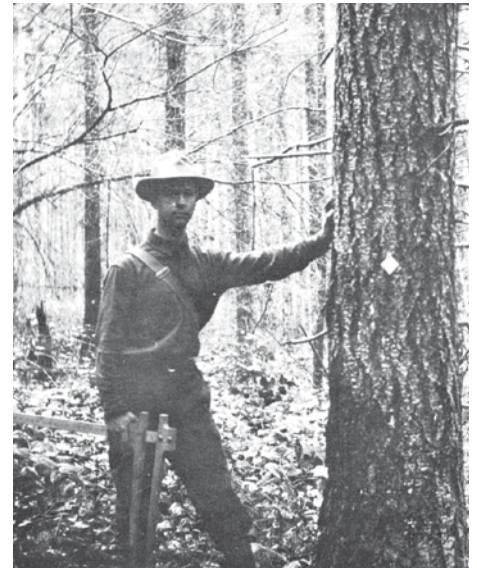
In the early days of the permanent study plot program, large calipers were used to measure tree diameter. Photo from USFS-PNW.
