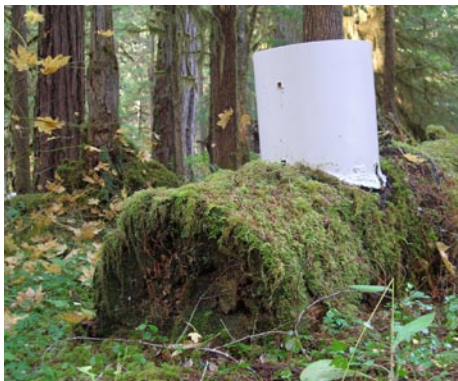
A decomposing Pacific Silver Fir ( Abies amabilis ) log with a respiration chamber used to measure carbon dioxide exhalation in Harmon's 200-year log decomposition experiment. Photo by Jay Sexton.
