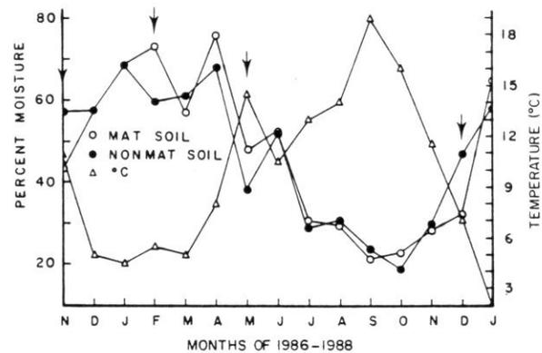
FIG. 1. Percent moisture and temperature (°C). Those months in which the differences between mat and nonmat soils were statistically different are indicated by arrows.
