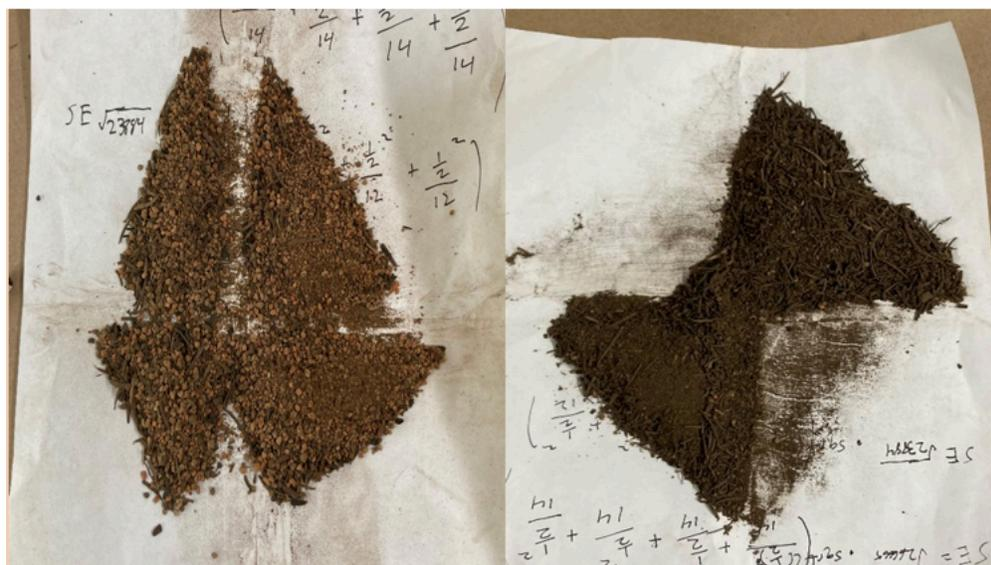
Figure 11. Splitting process used to obtain a 1-3 gram representative subsample for loss on ignition tests
