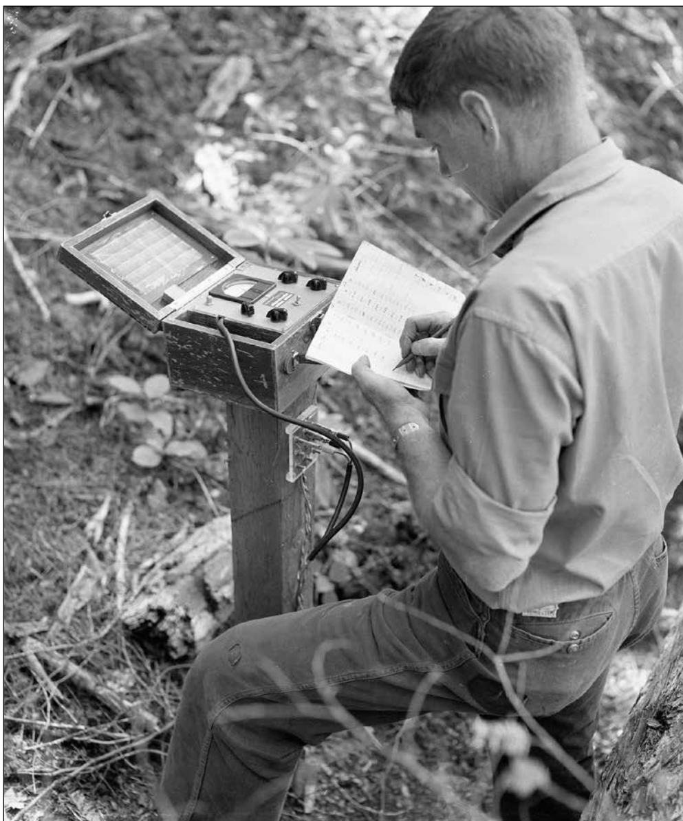
IN THIS 1961 PHOTOGRAPH, Jack Rothacher records readings from a soil-moisture meter station in Watershed 3 in the H.J. Andrews Experimental Forest.
