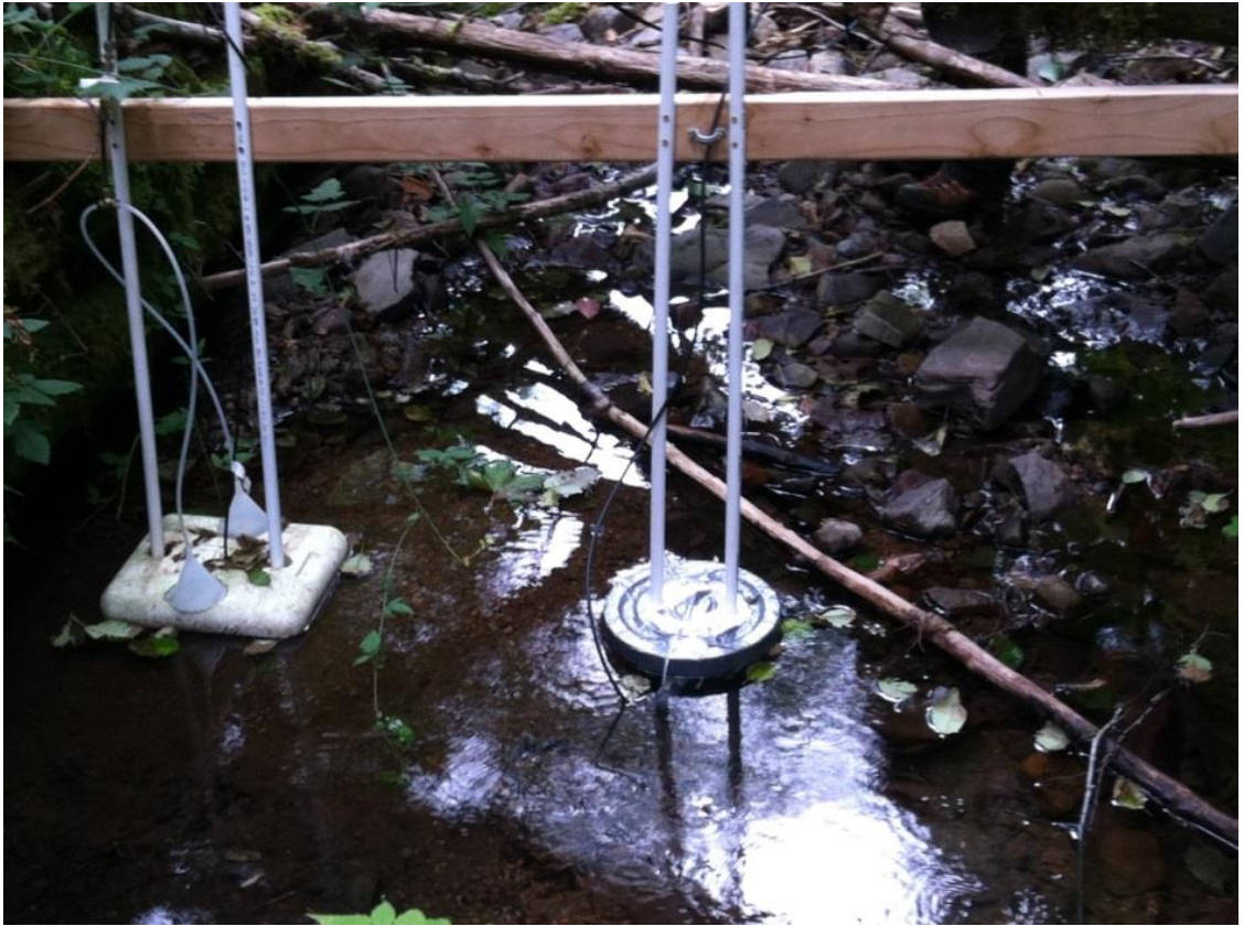
Figure C.12 - GMM deployed in the field. Probe is attached to Styrofoam float below the surface of the stream. The cable leads to the data logger in the logger box in Figure C.11
