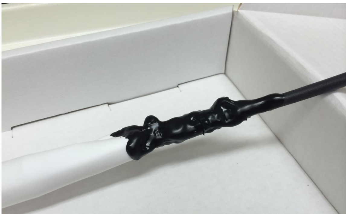
Figure C.9 - After the first layer is applied, allow the probe to dry in a well-ventilated area (i.e., fume hood) for 4-5 hours. Reapply an additional 3 to 4 layers of liquid tape in the same location. Make sure to look for bubbles or holes in the dry liquid tape. It is critical that there is a complete seal over the end of the probe. Once the 4 th or 5 th layer of liquid tape has been applied and given sufficient time to dry, the probe is ready for field deployment.
