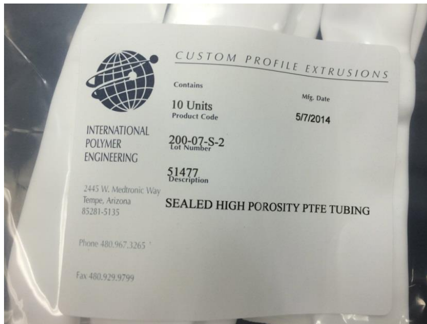
Figure C.3 - PTFE fabric used for the modification from International Polymer Engineering, Inc. This model is 200-07-S-2 and was sealed at one end like a sock.
