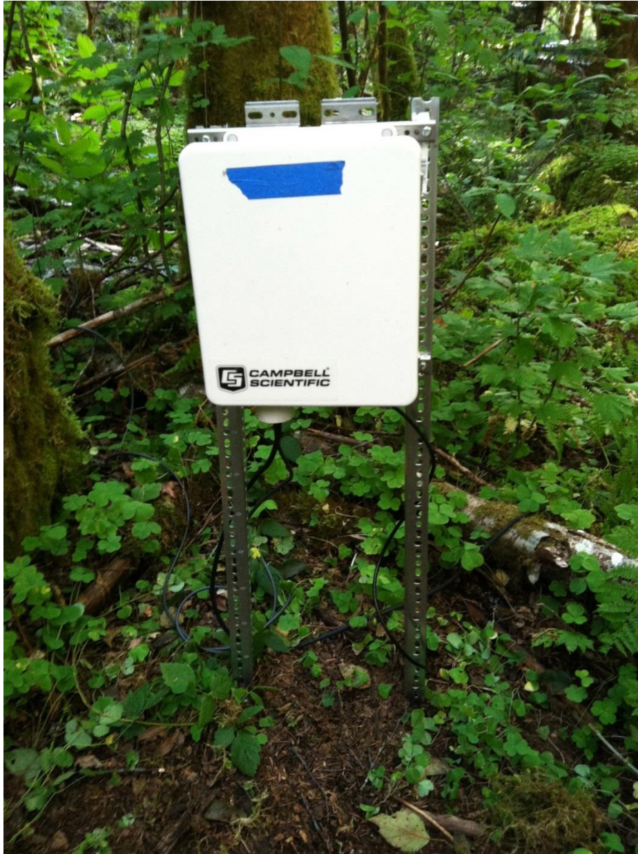
Figure C.11 - Data logger and GMM 220 deployed in the field. This box contains the data logger. Cables leaving the box lead to the probe and external power supply.
