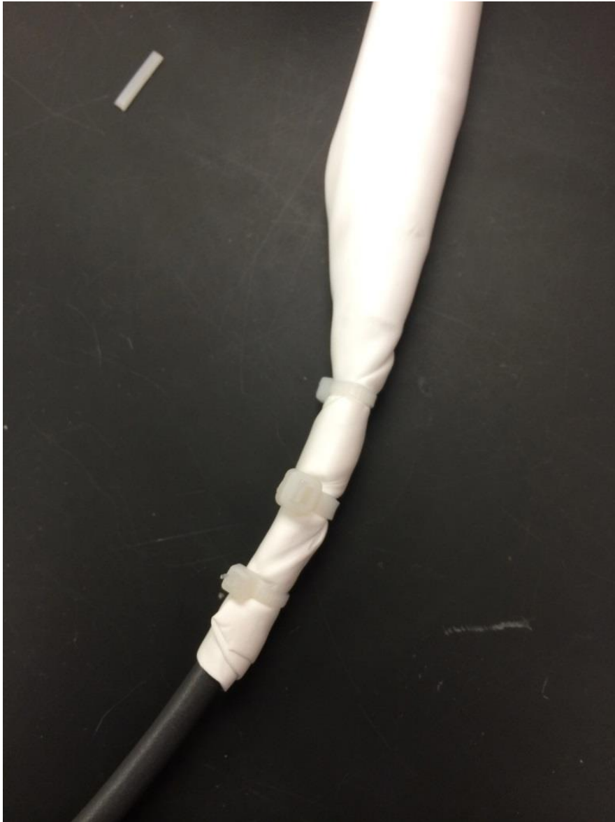
Figure C.6 - Trim the excess plastic from the zip ties. Make sure to be gentle with the PTFE tubing during this step – any abrasions or holes created may allow water to penetrate the sleeve and damage the sensor. If any holes in the PTFE fabric are identified, they must be patched during the next step of the modification process
