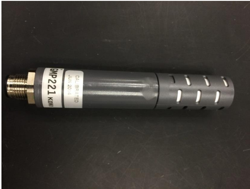
Figure C.2 - Close-up view of the CO 2 probe. The infrared sensor is housed within the vented section. This will be sealed by the PTFE fabric.
