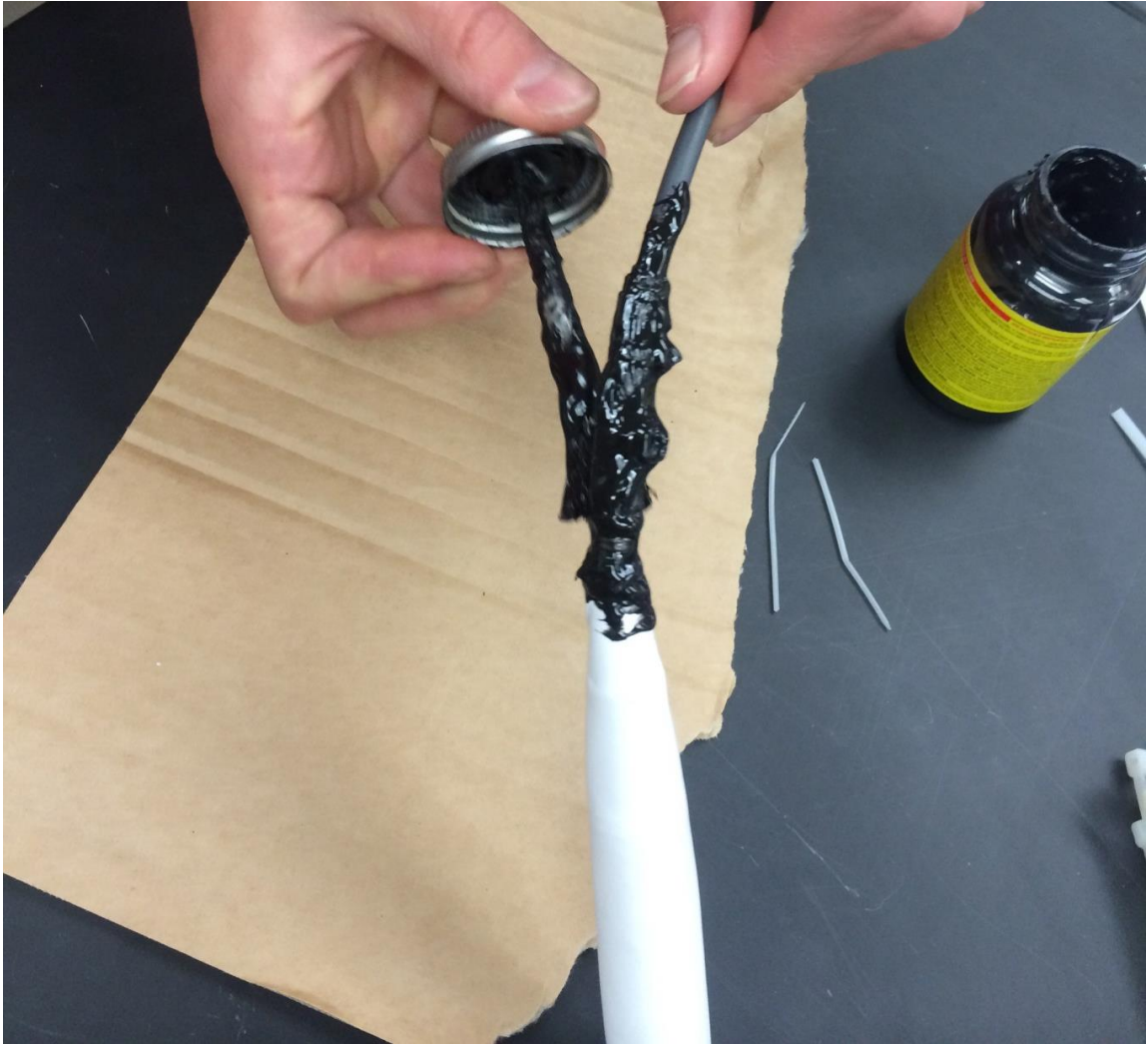
Figure C.8 - Apply the liquid tape above the zip ties and below the bottom of the PTFE. Look for any abrasions or rips in the fabric that require spot applications of liquid tape for waterproofing.
