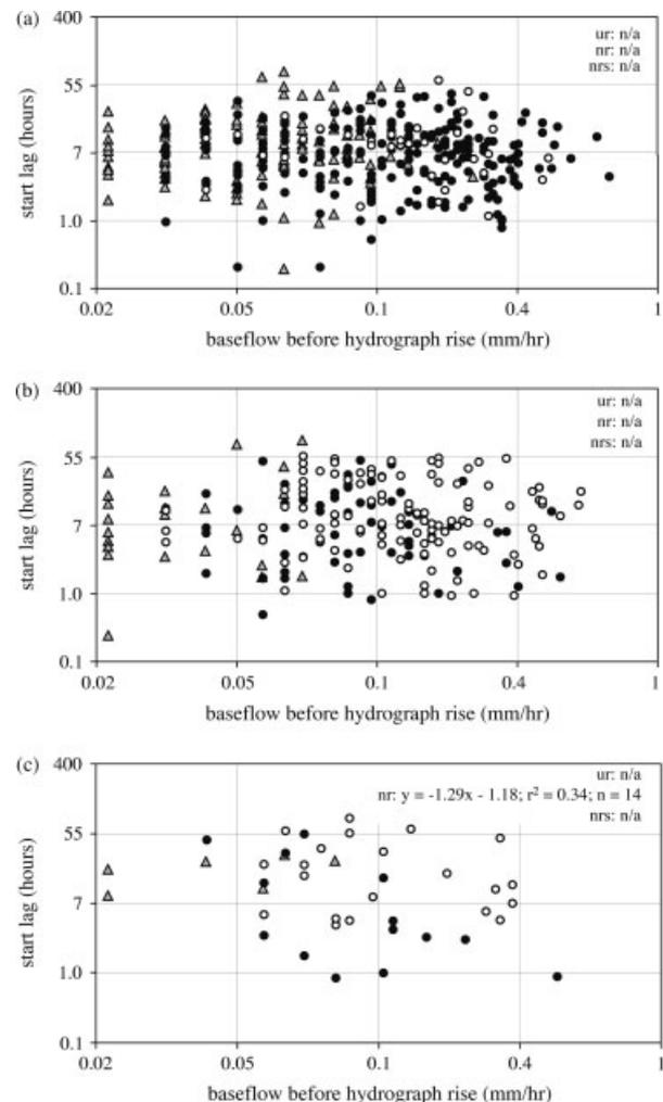
Figure 9. Relationships between baseflow before hydrograph rise ( $\text{mm h}^{-1}$ ) and start lag (h) for three event types in three watersheds: rain events on unsaturated soil ('ur', gray triangles), rain events on near-saturated soils ('nr', solid circles), and rain-on-snow events on near-saturated soil ('nrs', open circles), from (a) Watershed 9, 1969–1992; (b) Watershed 2, 1964–1992; and (c) Watershed 8, 1985–1992. Data were log-transformed for analysis and plotting
