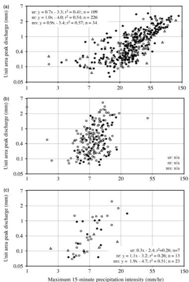
Figure 10. Relationships between maximum 15-min precipitation intensity ( $\text{mm h}^{-1}$ ) and peak discharge (mm) for three event types in three watersheds: rain events on unsaturated soil ('ur', gray triangles), rain events on near-saturated soils ('nr', solid circles), and rain-on-snow events on near-saturated soil ('nrs', open circles), from (a) Watershed 9, 1969–1992; (b) Watershed 2, 1964–1992; and (c) Watershed 8, 1985–1992. Data were log-transformed for analysis and plotting
