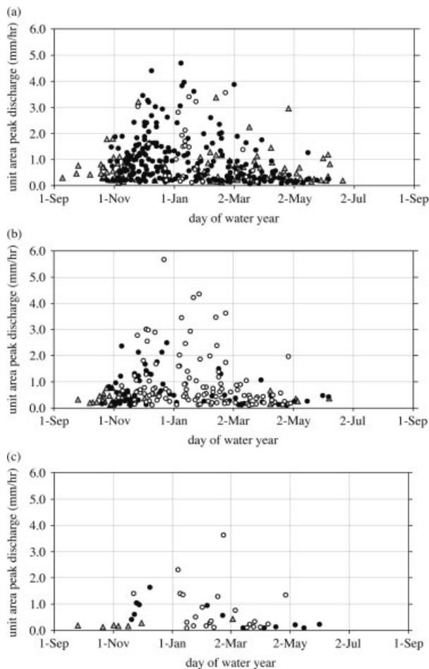
Figure 6. Unit area peak discharges ( $\text{mm h}^{-1}$ ) over the water year (1 October to 30 September) for three event types: rain events on unsaturated soil (gray triangles), rain events on near-saturated soils (solid circles), and rain-on-snow events on near-saturated soil (open circles), from (a) Watershed 9, 1969–1992; (b) Watershed 2, 1964–1992; and (c) Watershed 8, 1985–1992
