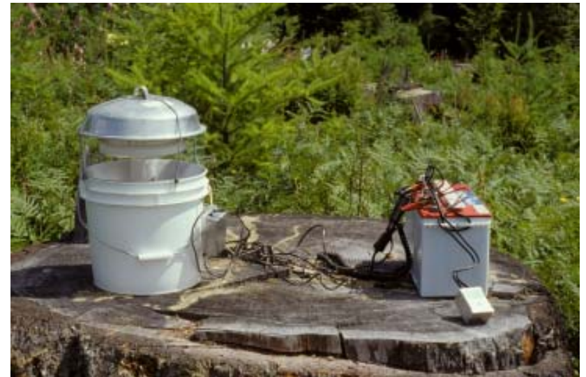
Figure 11 A light trap setup includes a containment bucket (a killing agent optional for unattended sampling), funnel, plastic veins holding the UV lightbulb, top fastened down with bungee cords, and electrical wires equipped with a photoswitch attached to a 12-volt battery. This setup can be used to sample night-flying moths for up to four consecutive nights.
