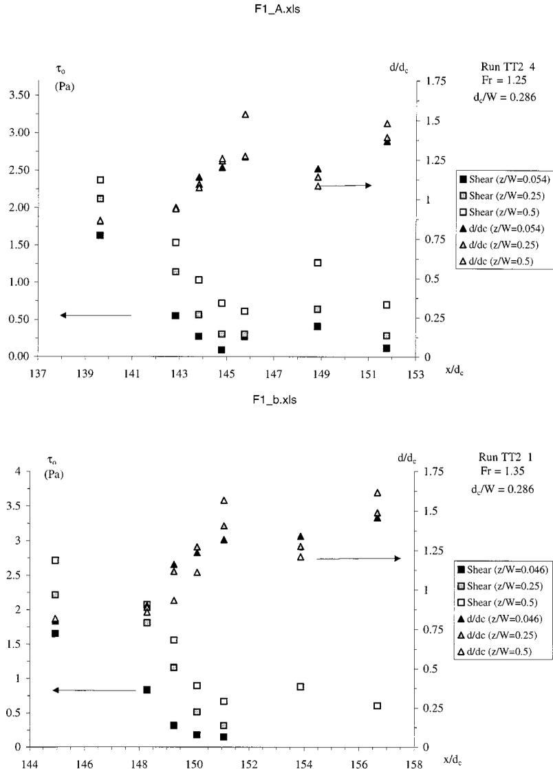
**Figure 1.** Bed shear stress along an undular hydraulic jump. (a) Flow conditions:  $Fr = 1.25$ ,  $d_c/W = 0.286$ ,  $W = 0.25$  m (Run TT2\_4). (b) Flow conditions:  $Fr = 1.35$ ,  $d_c/W = 0.286$ ,  $W = 0.25$  m (Run TT2\_1).
