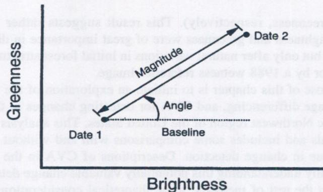
**Figure 6.2.** The concept of Change Vector Analysis in two spectral dimensions (adapted from Malila, 1980).
