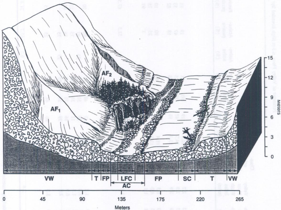
Fig. 4. Schematic diagram of valley floor surface types. Abbreviations used: LFC = low-flow channel; AC = active channel; FP = floodplain; SC = secondary channel; T = terrace; AF<sub>1</sub> = unincised, active alluvial fan; AF<sub>2</sub> = incised, inactive fan; VF = valley wall.
