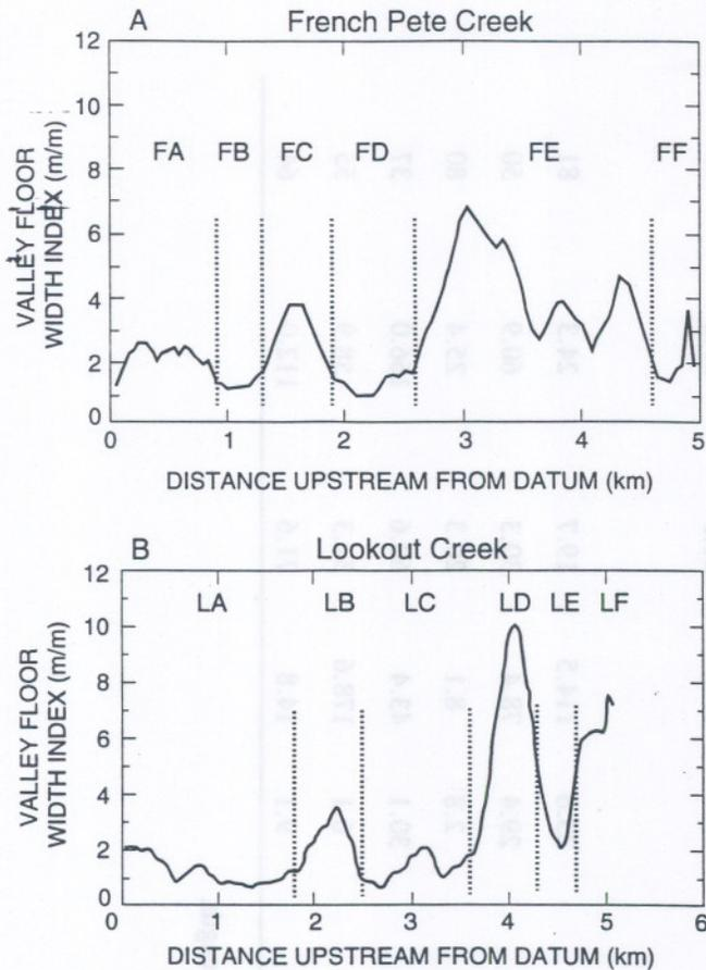
Fig. 5. Plot of valley floor width index (VFWI) as a function of distance upstream for the two study sites. VFWI was calculated as a 200-m running average of the ratio of active and floodplain widths to the average active channel width for the entire site, based on measurements of valley width taken at 50-m intervals. (a) Lookout Creek. (b) French Pete Creek.
