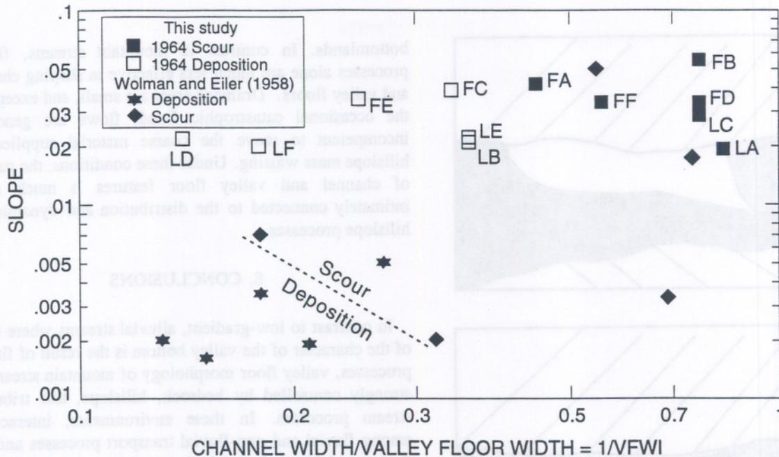
Fig. 9. Patterns of scour and deposition during floods in relation to channel gradient and the ratio of channel width to valley floor width, after *Wolman and Eiler* [1958]. Shown are Lookout and French Pete Creek reaches and data points for the Connecticut River following the 1955 flood. The dotted line is *Wolman and Eiler's* [1958] envelope curve (fitted by eye) distinguishing domains of scour and deposition for their data.
