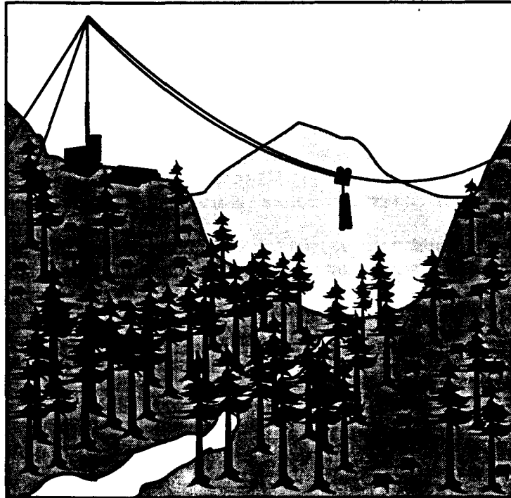
Figure 40. Yarding logs with full suspension across unharvested riparian management zone.
