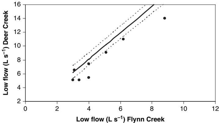
**Fig. 2.13** Regression between low flows on Flynn Creek and Deer Creek and posttreatment low flow observations
