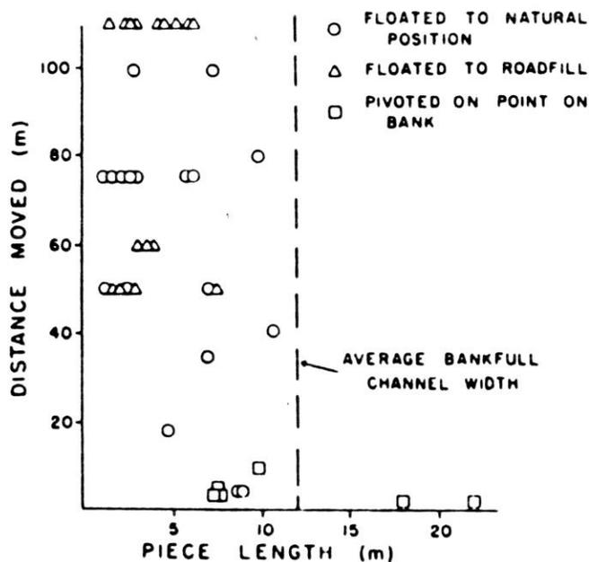
FIG. 3. Unanchored logs that were shorter than bankfull width were
