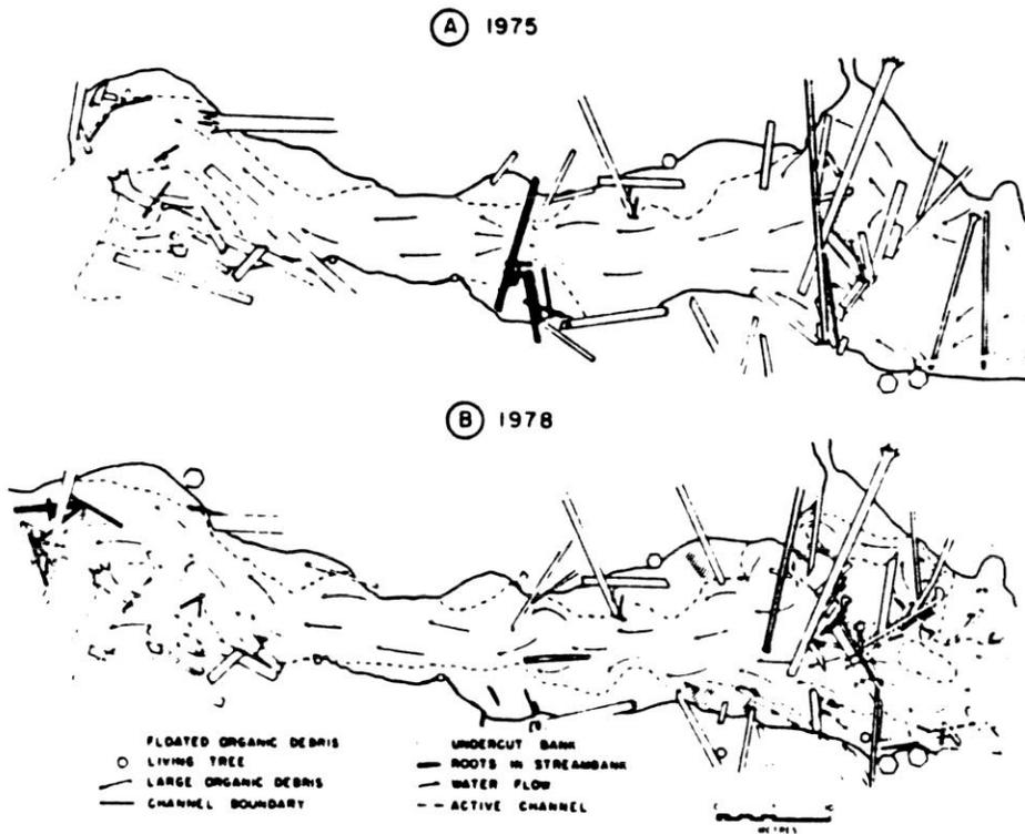
FIG. 2. The November 1977 high flow redistributed a large amount of wood in Mack Creek. For example, most of the material highlighted in black (A) was washed out of the study area, but some material was redeposited at the next bend (black pieces in B). The stippled log in A broke and pivoted downstream.
