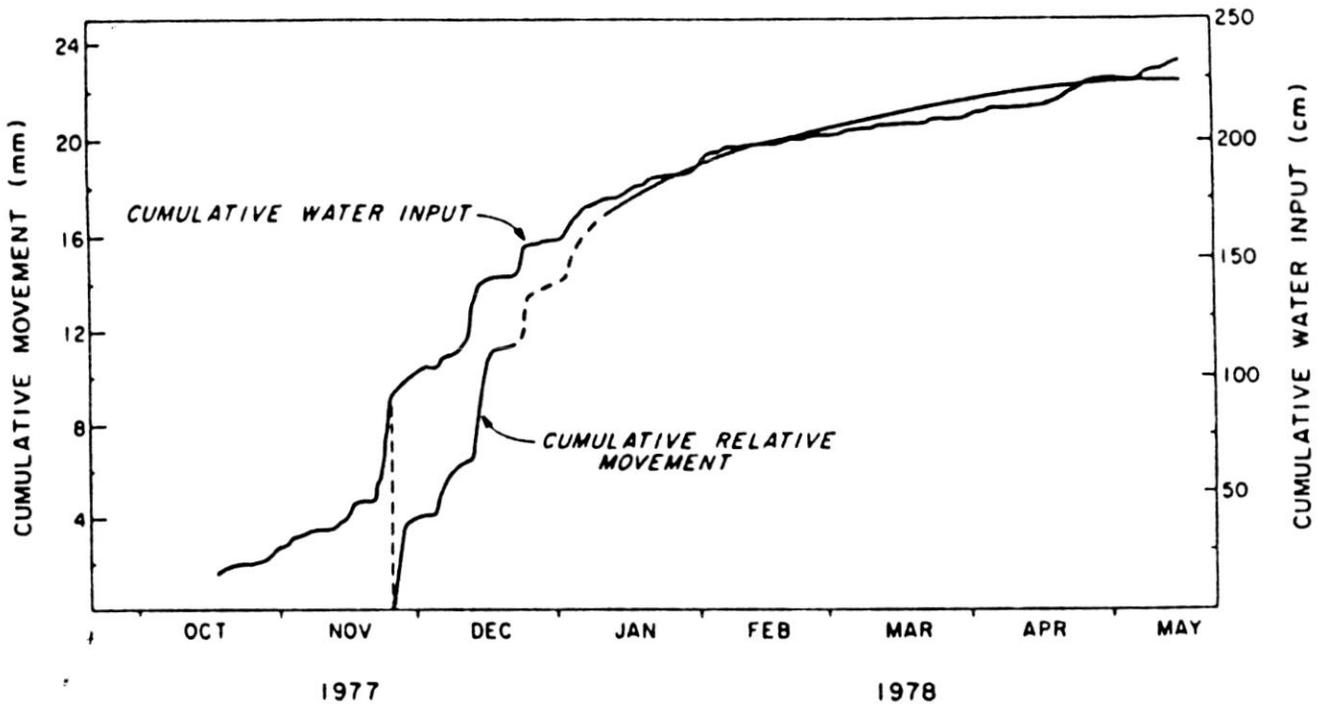
Figure 3. Cumulative water input and relative movement at crackmeter located at site 6 (Fig. 2). Movement curve is dashed for period when only total movement is known.
