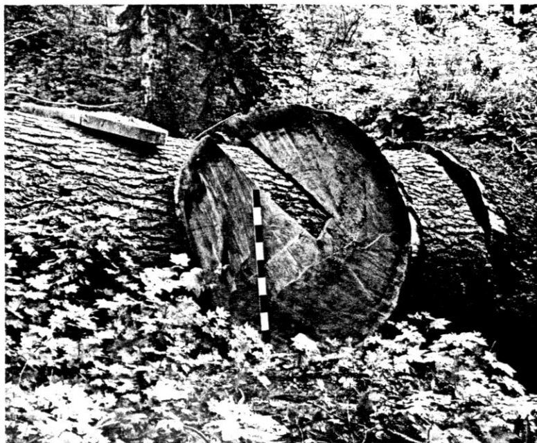
Figure 7.--Large transverse disk from sectioned noble fir with the representative radius removed.
