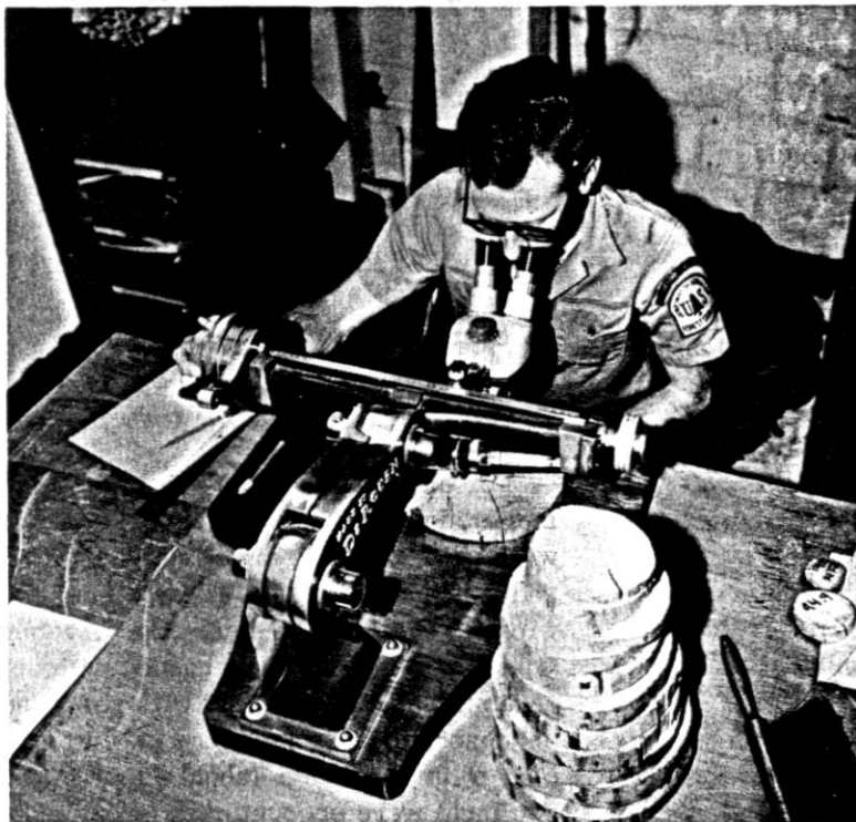
Figure 10.--A dendrochronograph was used to measure radial growth where annual rings were closely spaced.
