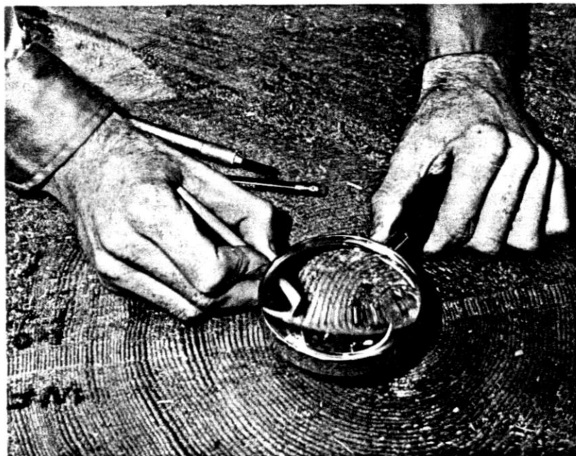
Figure 6.--Ring counting using large reading glass.
