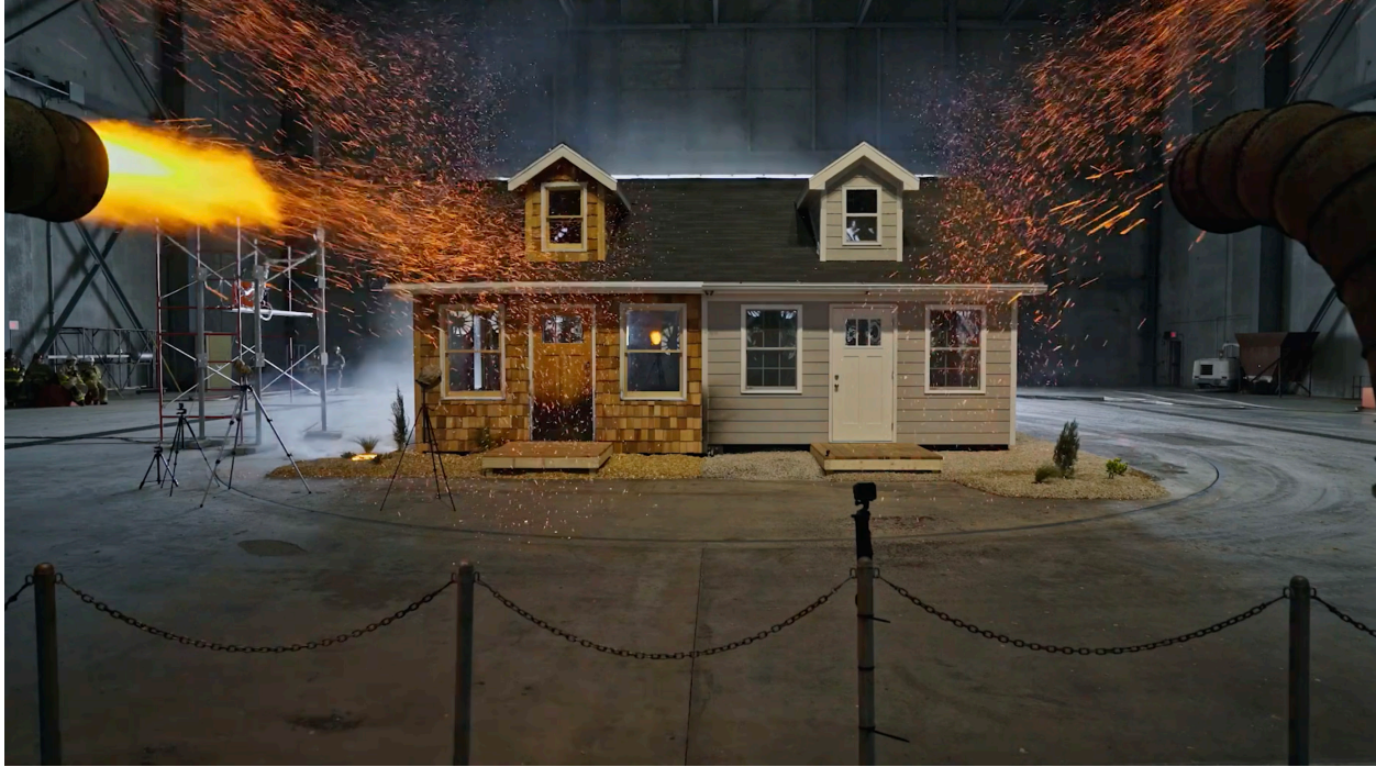
Figure 4. Testing resistance of home building and landscaping materials to ignition from wind-blown embers. Photograph courtesy of ElementalFilm.com.
