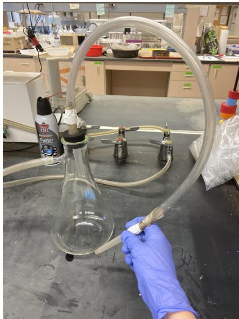
Fig. 6 Aspirating materials: aspiration tube and 1000 mL Erlenmeyer sidearm flask connected to bench vacuum.
