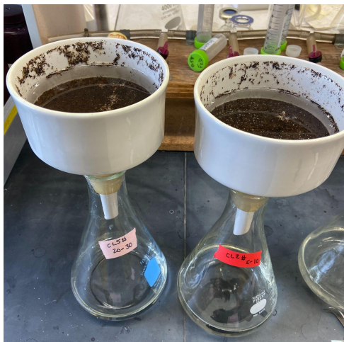
Fig. 8 Twelve cm ID porcelain Buchner funnel containing a 110 mm glass fiber filter seated atop a 1000 mL Erlenmeyer sidearm flask connected to a vacuum funnel. This contained LF of the control sample for low burn severity, replicate 5 (“CL5”, left) and paired control soil sample for low burn severity, replicate 2 (“CL2”, right).
