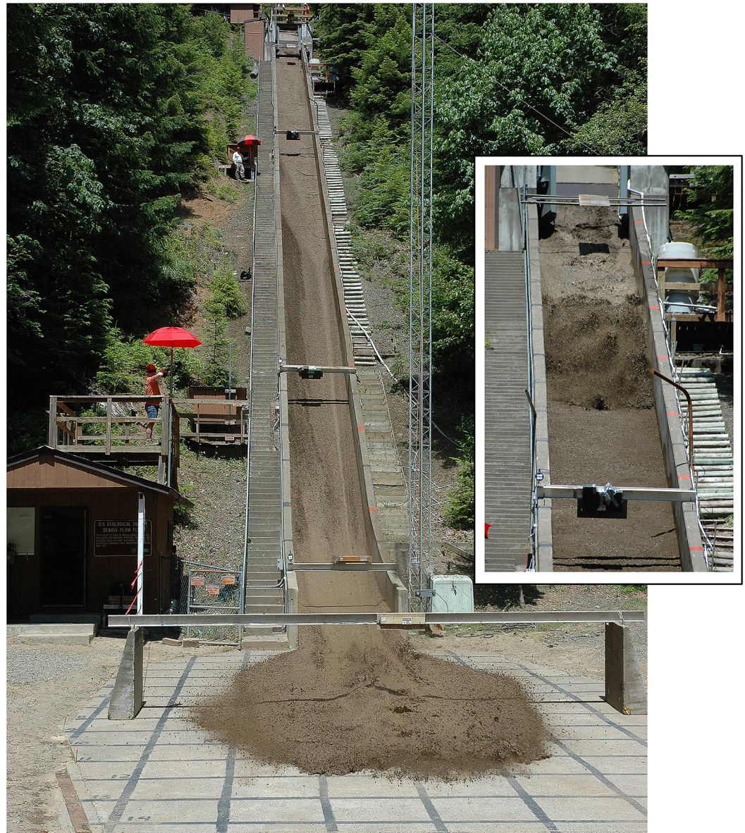
Figure 2. Photographs of a USGS debris flow flume experiment in which a debris flow entrained wet bed sediment that partially liquefied as it was overrun. Inset photo shows a close-up view of the agitated flow front interacting with bed sediment about 15 m downslope from the flume head gate. USGS photos by Matthew Logan, 21 June 2007.
