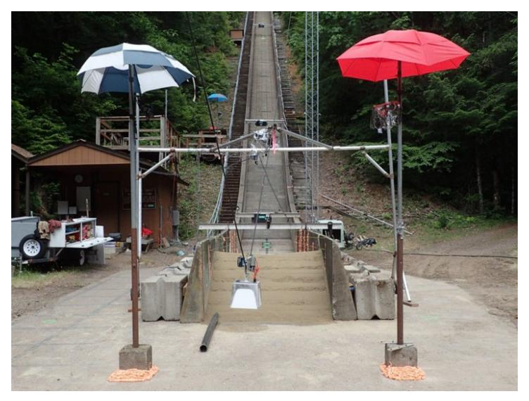
The U.S. Geological Survey's (USGS) 95-meter-long debris flow flume facility is located near Blue River, Ore., in the H.J. Andrews Experimental Forest. As seen here in June 2018, the flume is heavily instrumented during experiments, including with 4K video cameras (under the umbrellas and in the mobile, remotely controlled white box) and multiple digital still cameras with synchronized shutter releases to enable photogrammetry. Credit: USGS
