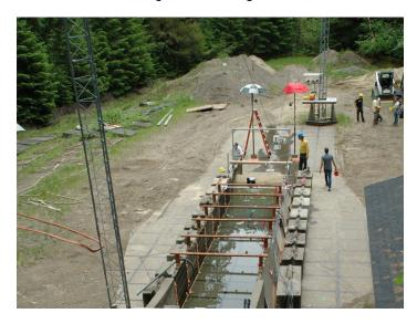
The filled pond setup with an earthen dam at the far end is seen in late May 2019 shortly before an experimental debris flow was released. Credit:
