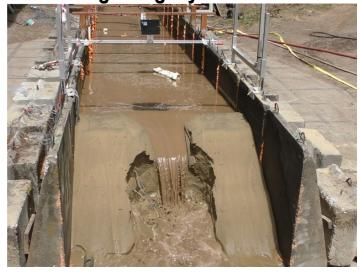
During an experiment in early June 2019, the earthen dam blocking the pond failed as a result of a debris flow displacing the water in the pond and generating a tsunami. Instrumentation used to document the experiment included sonic sensors (mounted on wooden crossbeams) for wave height detection, a depth camera (mounted on an aluminum crossbeam) to capture dam erosion, pressure plates (not visible at the base of the pond), and pore pressure sensors throughout the dam (not visible). Credit: USGS
