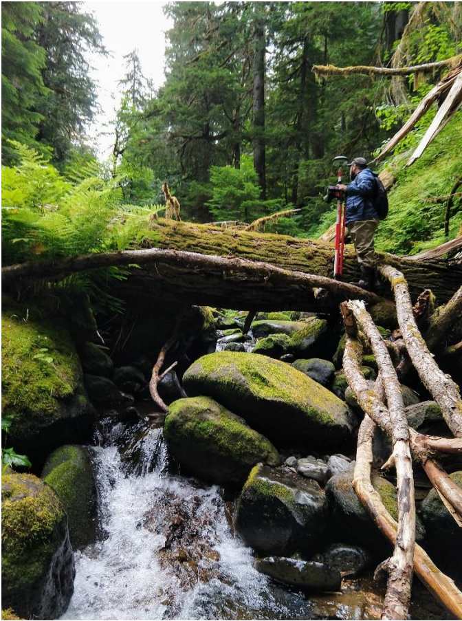
Figure B.6: Field assistant holding RTK GPS unit above channel spanning logjam at Mack Old Growth near cross section MAC07
