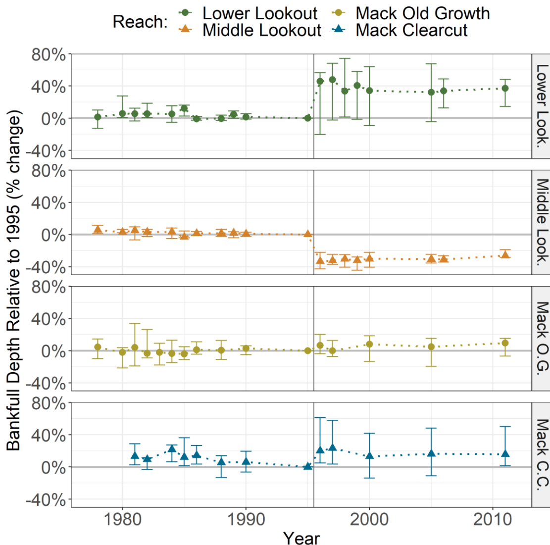
Figure 9: Bankfull depths as a ratio relative to the 1995 values at each reach. Median values represented by dots and interquartile range represented by bars. Values above 1 indicate that bankfull depths deeper than those in 1995 while values below 1 indicate bankfull depths shallower than those in 1995. Median bankfull depths in Lower Lookout and Mack Clearcut increased after the flood of 1996 although both reaches displayed a wide range of post-flood variability. Median bankfull depths at Middle Lookout became shallower following the flood of 1996.
