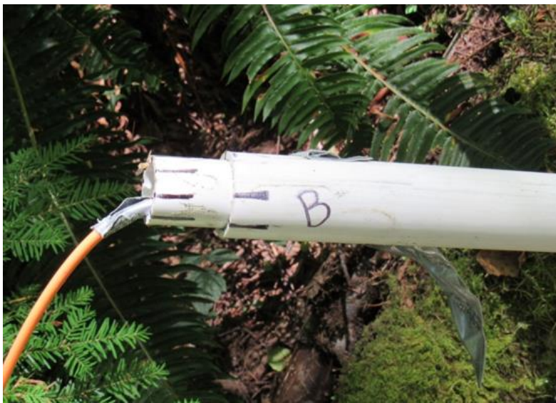
Figure 59: Deployed Vaisala probe in outer PVC casing.
