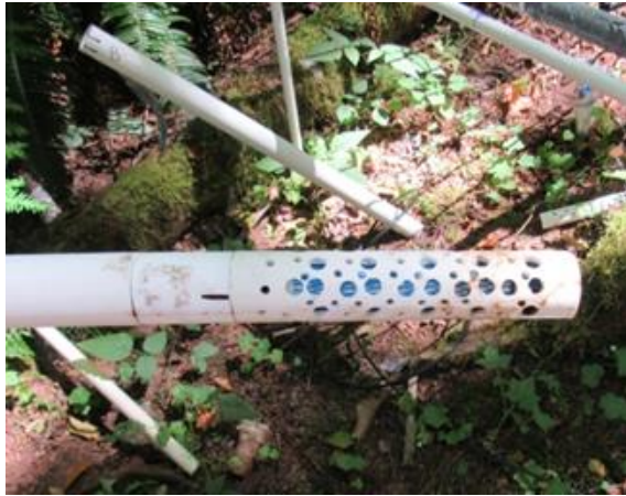
Figure 57: Vaisala probe in PVC casing.
