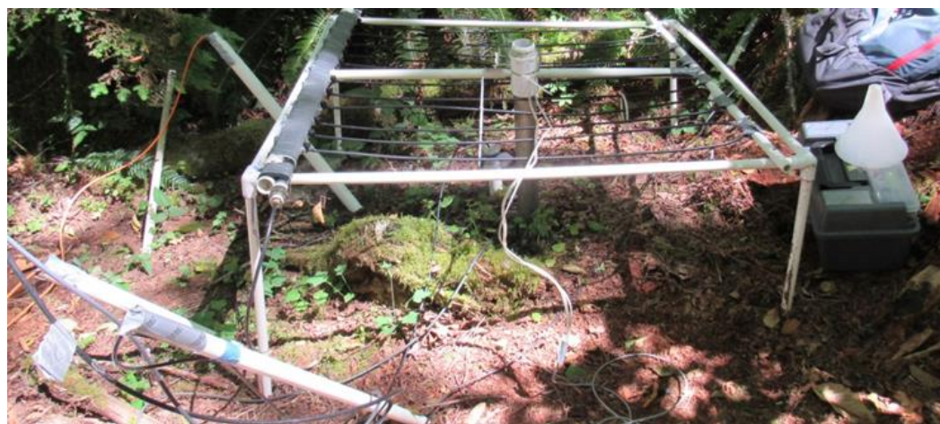
Figure 56: Two additional views of study column and experimental rain simulator.
