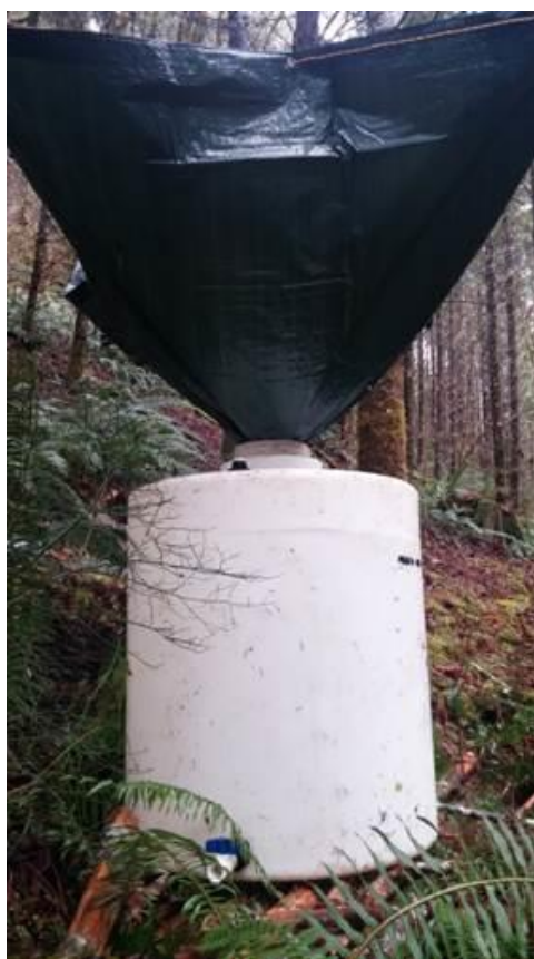
Figure 63: Rain collector close-up.
