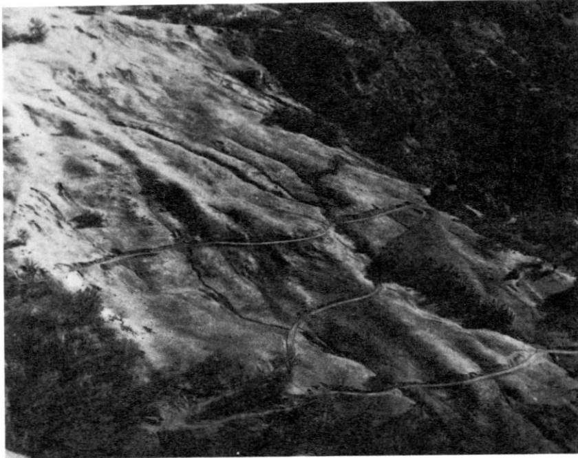
Figure 2. An example of creep and slump-earthflow processes on forest lands in northern California, U.S.A. The entire slope is undergoing creep deformation, but note the discrete failure (slump-earthflow) marked by the steep headwall scarp at top center and the many small slumps and debris avalanches triggered by surface springs and road construction.
