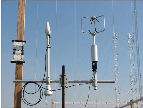
Figure 2.1: Photo of a SUSAN unit at the Botany and Plant Pathology site. The sonic anemometer is attached to the right and the thermohygrometer to the left side of the metal crossbar.
