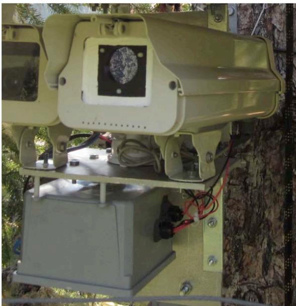
Figure 3: The camera was contained in a fan-ventilated housing. The camera's lens was embedded in a black Delrin baffle machined to fit in the front of the camera housing. The baffle was equipped with a germanium window that had a coating designed to maximize its transmissivity in the 8 -12 \mu\text{m} spectral range.
