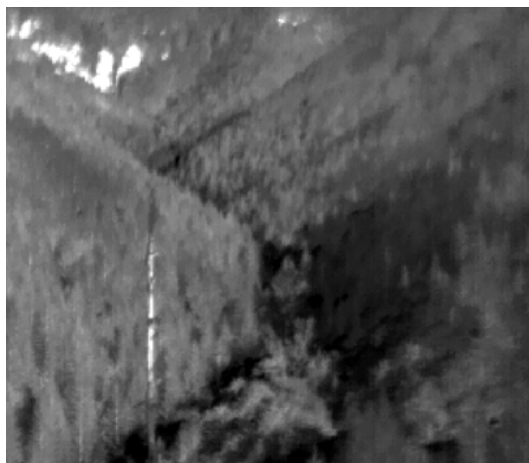
Figure 28: The thermal images acquired deciduous and non-deciduous trees, branches and tree trunks, rocks, and soil. All of the items have unique thermal properties. The emissivity for each item differs in the 7.5 \mu\text{m} to 13 \mu\text{m} range. The bright rocks in the top left of the image illustrate this point. The bright tree in the foreground also shows the effects of differing emissivities on the image. Additionally, the tree is not actually in Watershed 1.
