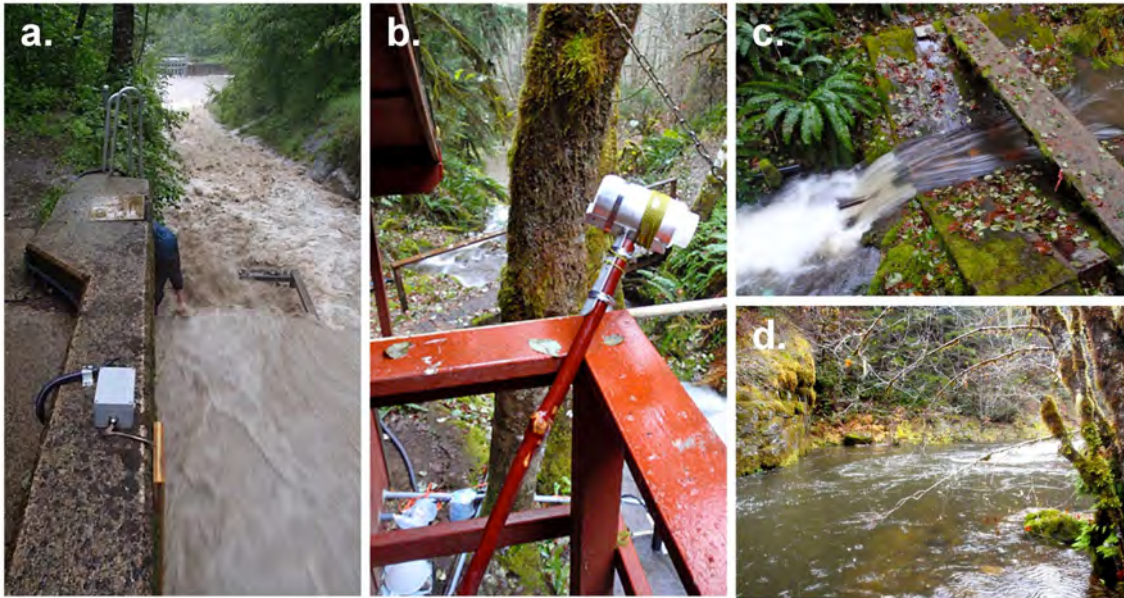
Figure 3.1: Suspended sediment sampling. (a) Sampling in the Erlenbach at peak flow of the 29 July event. (b) Sampling bottle and bottle holder used in Oregon to make sampling safer and ensure clearance of stream banks. (c) Watershed 1: falling limb of the 21–22 November event. (d) Lookout Creek: falling limb of the 16–17 November event.
