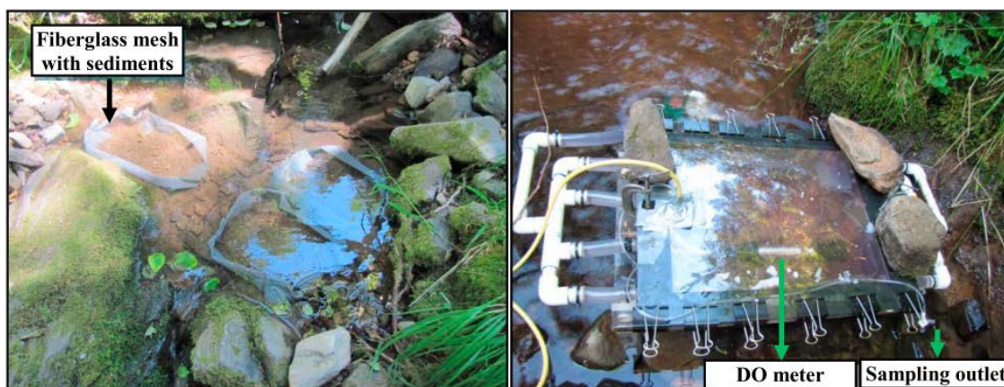
Figure 4.3. Respiration chamber experiments conducted at the H.J. Andrews Experimental Forest to test the correlation between \Delta Rru and \Delta DO . Left) fiberglass incubation meshes. Right) recirculating chamber with incubated sediments.
