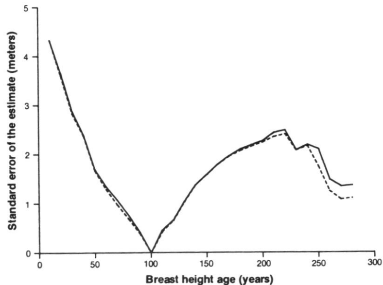
Figure 8.—Standard error of the estimate (uncorrected for the degrees of freedom in the models) for site index models by decadal age. The solid line is for the final site index model, equation (14), and the dashed line is for the regressions produced by Heger's (1968) method, equation (7).
