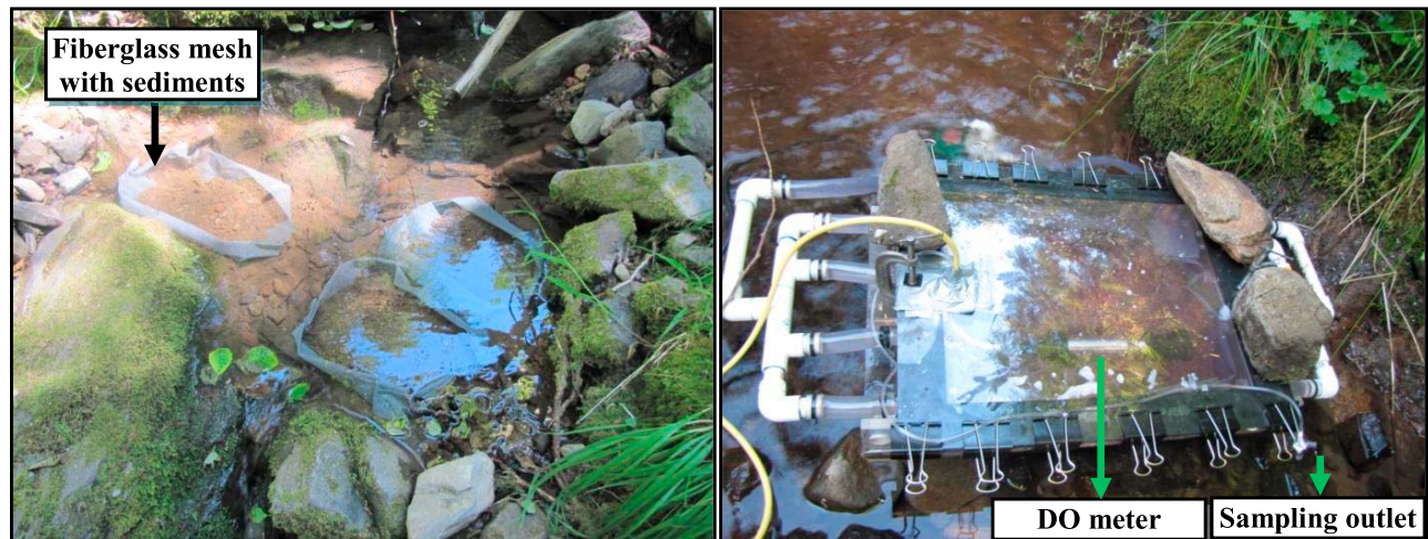
Figure 3. Respiration chamber experiments conducted at the H. J. Andrews Experimental Forest to test the correlation between \Delta Rru and \Delta DO : (left) fiberglass incubation meshes; (right) recirculating chamber with incubated sediments.
