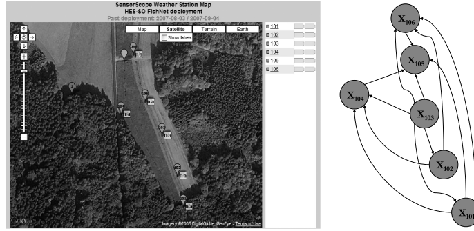
Fig. 6. Left: top-down view of the FishNet Deployment. Right: learned dependency relationships among the six sensor stations at the deployment.
