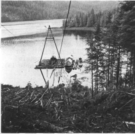
Figure 11.--A-frame skidders, such as this one operating in Traitors Cove in 1957, are used to log direct to a protected beach. Such operations are less common today, accounting for about 2 percent of the total log production.
