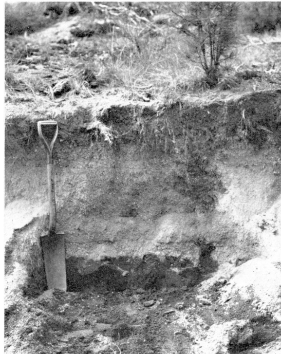
FIG. 4. Lapine soil profile. Note the dark-colored A1 and AC surface horizons, the lighter-colored gravelly C horizons, and the abrupt boundary to the underlying buried soil.
