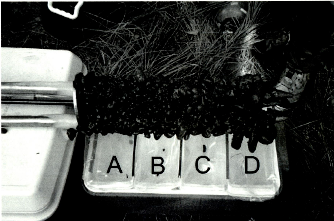
Figure 3: Freeze core showing 11.5 cm bins lined with plastic and marked by relative depth (A-D).
