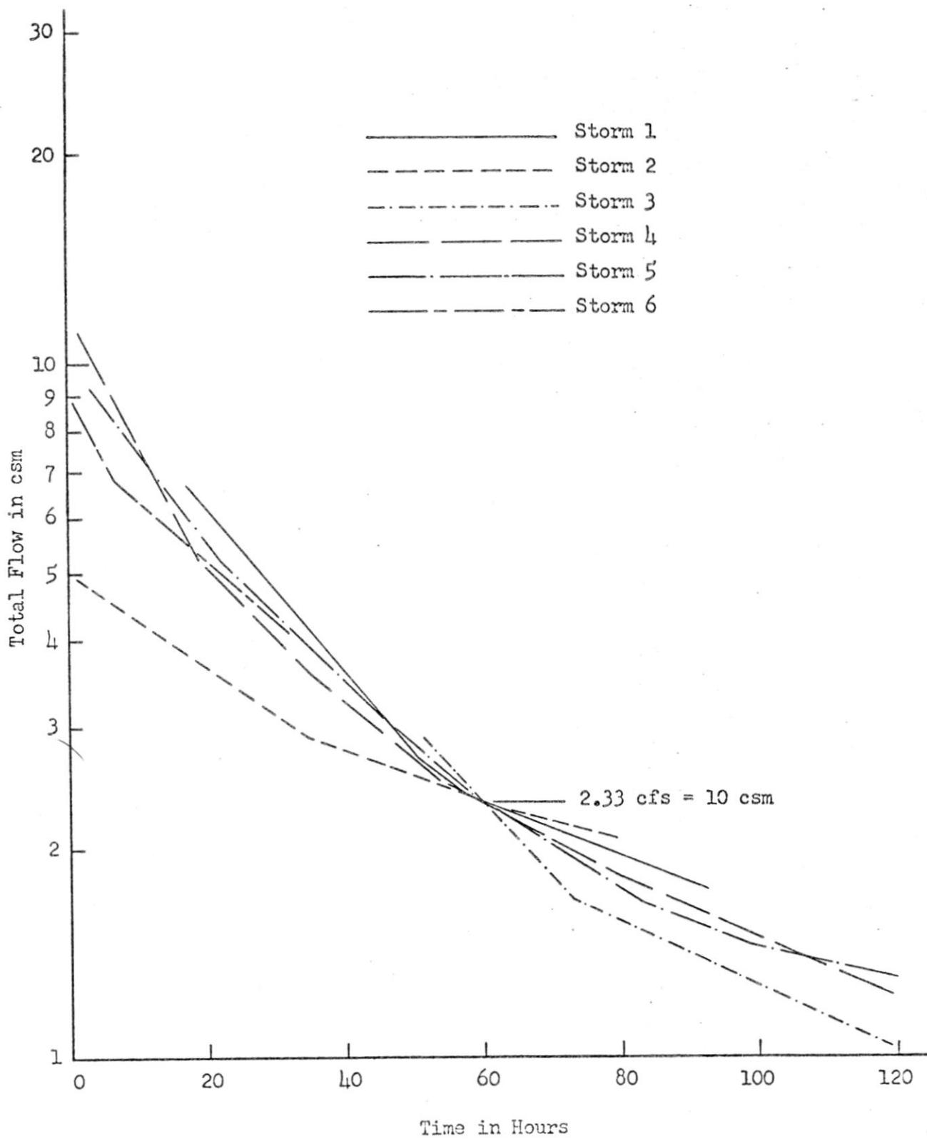
Figure 12. Hydrograph recessions of Watershed #3.
