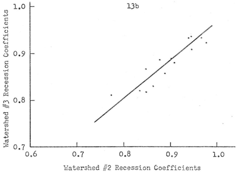
Figure 13. Comparison of six hour recession coefficients.
