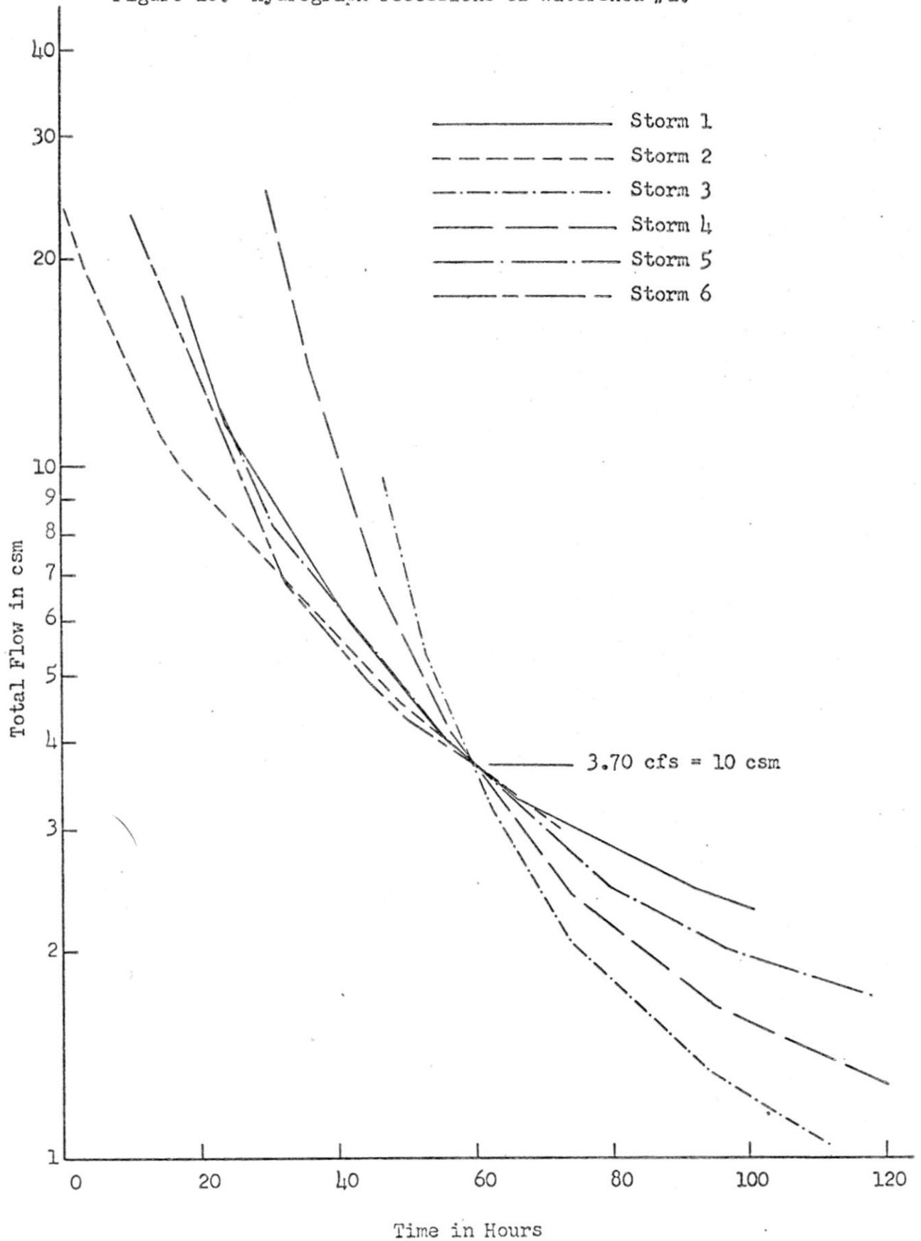
Figure 11. Hydrograph recessions of Watershed #2.
