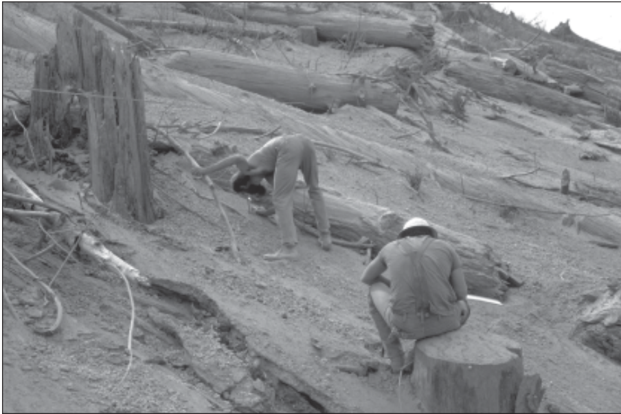
Figure 36—Fred Swanson (left) takes initial readings from a set of erosion pins established in August 1980 at a study site on Mount St. Helens, shortly after the eruption earlier that year.
