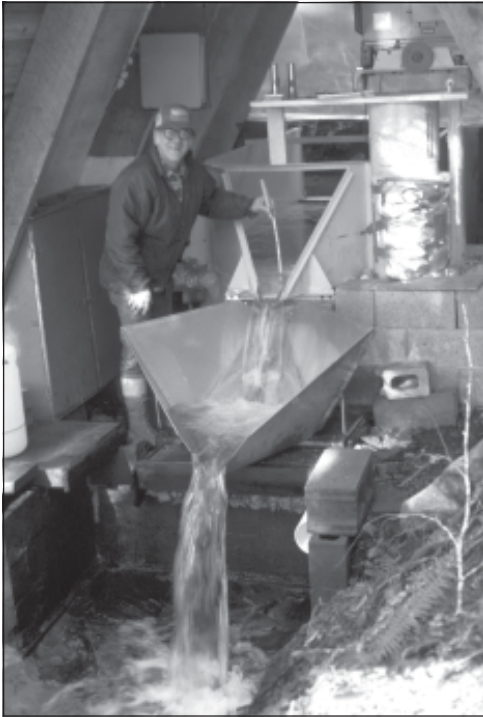
Figure 32—An early pattern of long-term, continuous data collected in a consistent fashion was an established tradition by the time Roswell (Ross) Mersereau made these measurements of streamflow in Watershed 6 at a gaging station equipped with a 2-foot H-flume and the venerable Stevens A-35 recorder on which the group relied for consistent data comparable across multiple decades.
