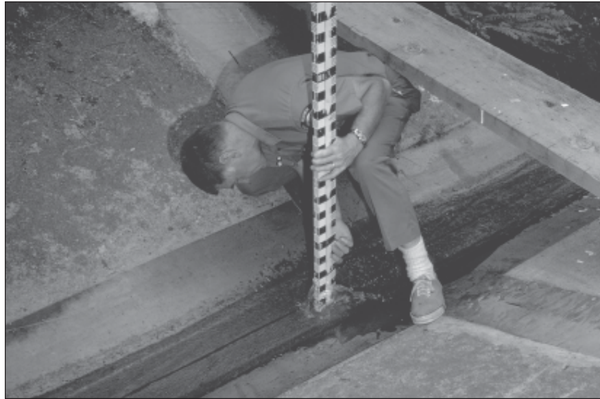
Figure 17—Among his other responsibilities, Jack Rothacher maintained long-term watershed records at the experimental forest. This photo shows Rothacher making stream discharge measurements at one of the three small watersheds (WS 1, 2, 3), by using a velocity head rod. This method was used to calibrate these 120-degree, trapezoidal flumes.
