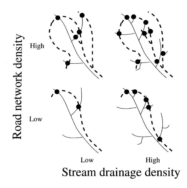
Figure 5. Schematic examples of road (dashed line) and stream (solid line) networks of high and low densities, showing highest density of road-stream intersections (dots) and, therefore, potential interactions in watersheds with high densities of both roads and streams.
