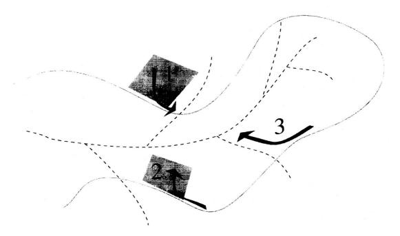
Figure 1. Types of network-patchwork interactions involving roads. Material (e.g., water, sediment), organisms (including propagules), and energy can move from vegetation patches to segments of a road network (1), from road segments to vegetation patches (2), and between road and stream networks (3).
