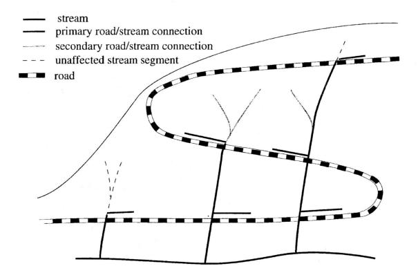
Figure 4. Effects of roads on stream and riparian networks include road ditches serving as extensions of the stream network and effects of streams and associated materials (e.g., sediment) on road segments encountered along the flowpath. The extent of stream network potentially affected by road influences can be expressed in terms of direct and potential influences and in terms of percent of network length affected and in terms of percent extension of drainage network density.
