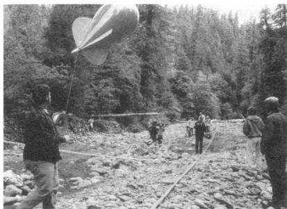
Fig. 6. Terrestrial-aquatic interactions are a major theme of research at the Forest. A small, hand-lined blimp with camera is being used to record channel changes and disturbance to riparian vegetation caused by a large flood. Photograph by Pam Druliner.
