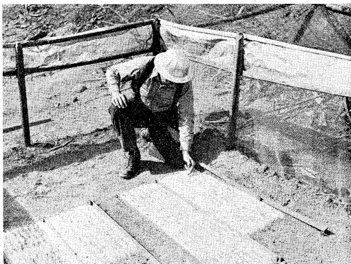
Artificial seedbed study was made to explore ways of overcoming seedling losses due to hot seedbed conditions. Seedbeds shown above were white silica sand of different size particles. Other seedbed materials included basalt gravel, mineral soil, needle litter, vermiculite, and charred surface material.
