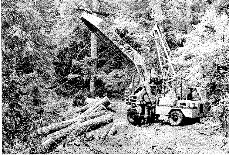
The mobile yarder-loader machine used for salvage logging in old-growth residual stands.
