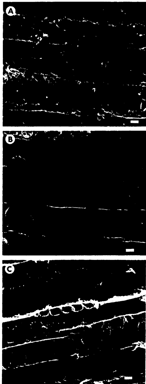
FIG. 2. SEM of wood samples from the study log. (A) Exposed side of a surface scraping, (B) underside of a surface scraping, and (C) core sample from a 25-cm depth. Bars, 10 \mu\text{m} .
