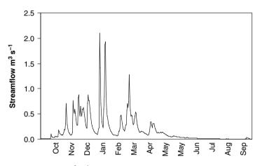
Fig. 2.2 Daily streamflow (m<sup>3</sup> s<sup>-1</sup>) for Flynn Creek Water Year 1972
