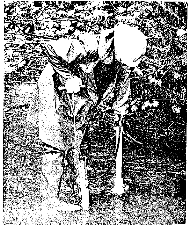
Figure 10. Pumping water from a standpipe under 1-inch head to determine permeability of intragravel environment.
