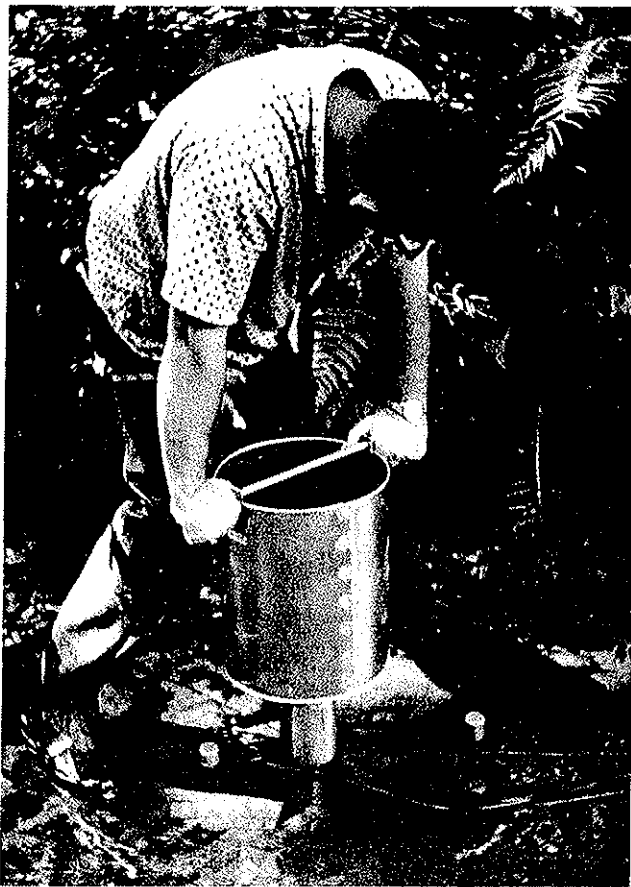
Figure 8. Inserting the Gravel Sampler into Spawning Gravel in Deer Creek.
