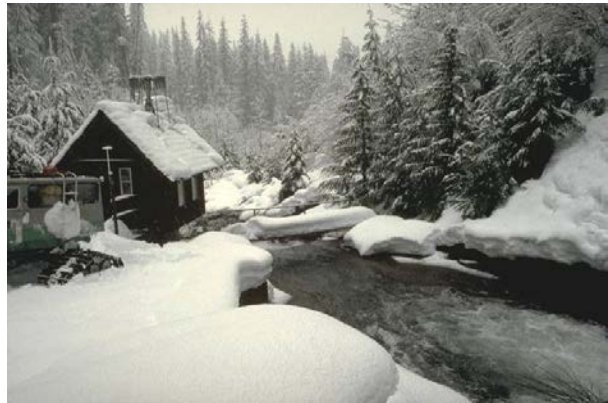
Mack Creek gaging station with heated orifice raingage and windshield on roof. (Al Levno 1989)
