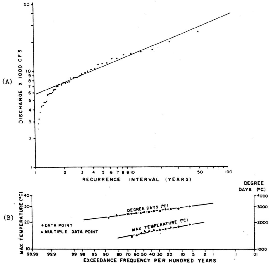
Fig. 2. North Santiam River (5th order), Oregon, recurrence intervals for maximum yearly floods (A) and temperature (B) based on a 20 year record. Degree days calculated as mean daily temperature times number of days having that mean and summed over the water year (October 1 - September 30). Recurrence interval ( $T_R$ ) =  $\frac{1 + n}{m}$ ,
