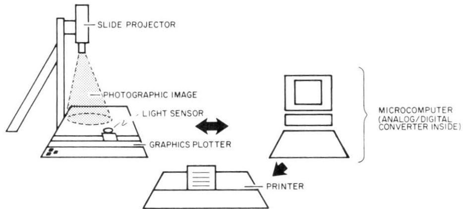
FIGURE 2. Schematic of the automated fisheye photographic analysis system.
