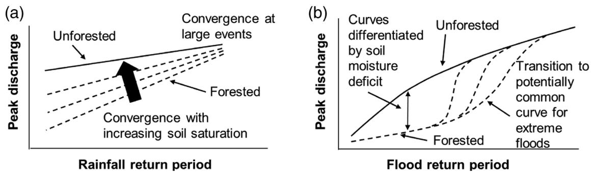
**FIGURE 7** Conceptual comparison of peak discharges for forested and unforested catchments as a function of (a) rainfall event return period (chronological pairing) and (b) flood return period (frequency pairing)
