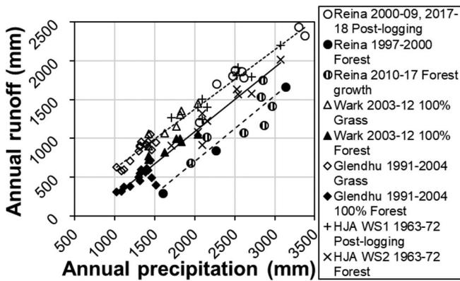
**FIGURE 4** Comparison of annual runoff with annual rainfall for the four sites. Data are separated into three alignments characterized by fitted linear trendlines, as described in the text
