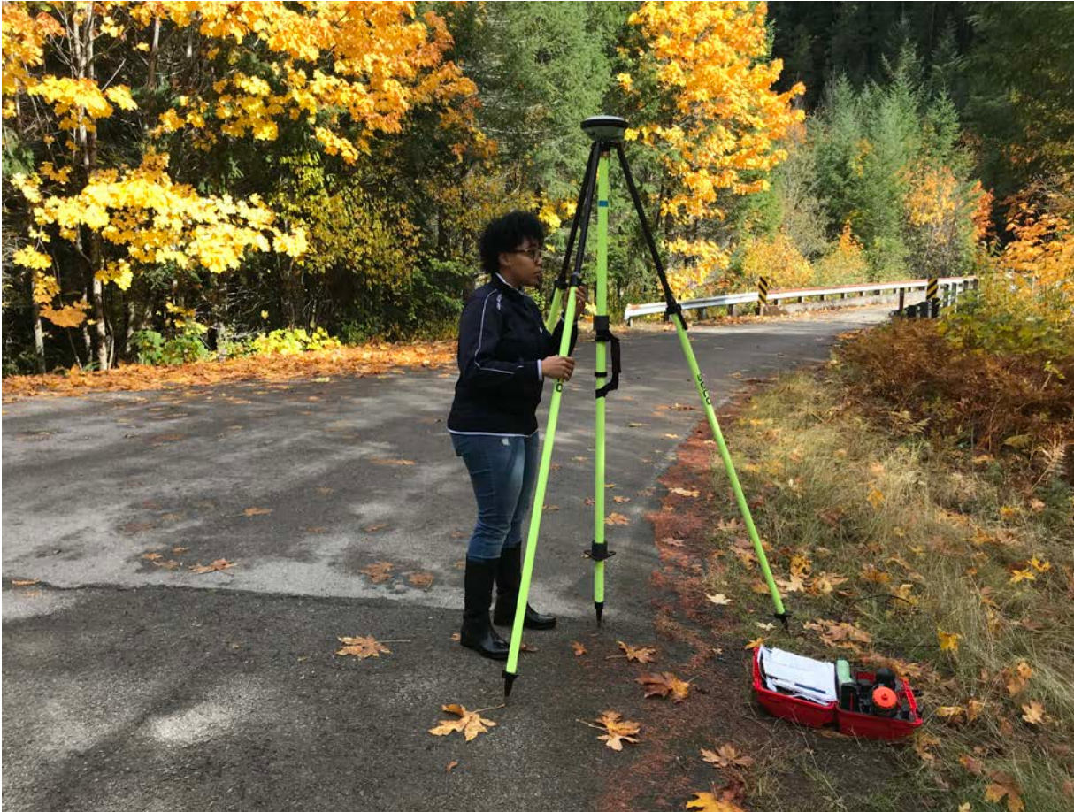
Figure 3.14: Fatima Taha setting up the Leica GS14 GNSS receiver at CP006 for collection of rapid static data on October 24th, 2017.
