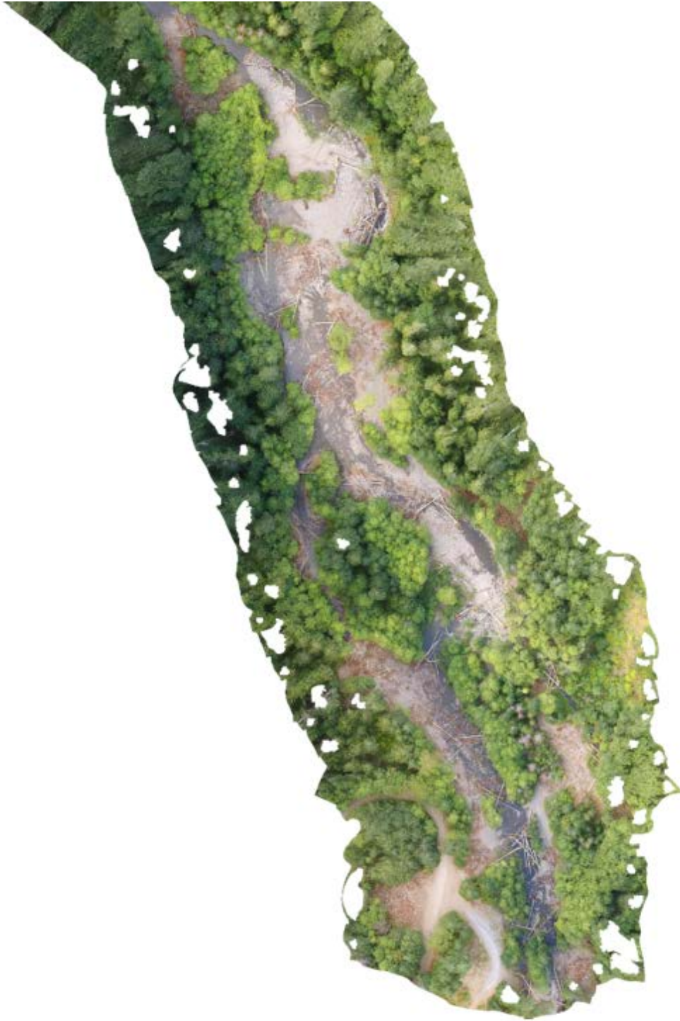
Figure 3.12: Orthomosaic of Deer Creek at Site 4 in September 2016, immediately after Stage 0 restoration was completed. Created with 237 UAV-captured aerial images.
