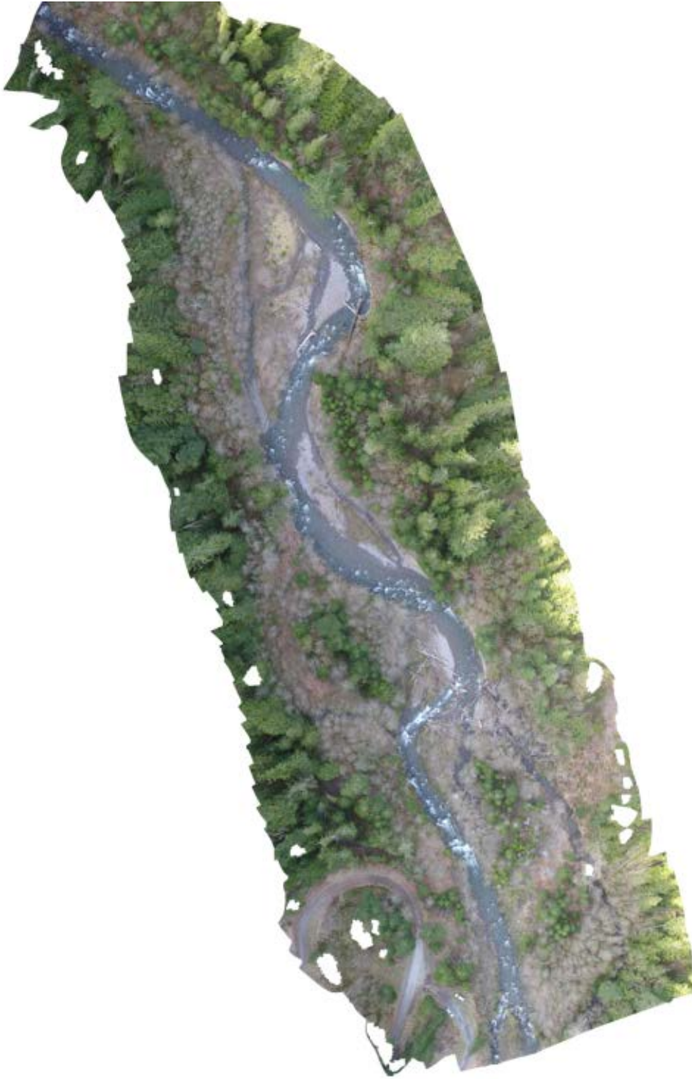
Figure 3.11: Orthomosaic of Deer Creek at Site 4 in April 2016, before Stage 0 restoration was completed. Created with 217 UAV-captured aerial images.
