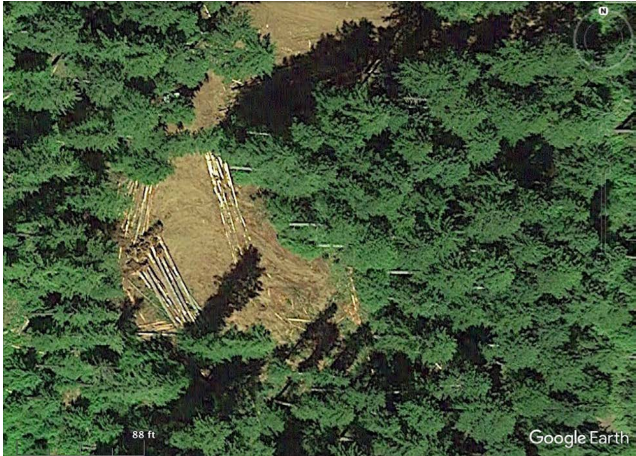
Figure 3.7: Upland stand gap for large wood procurement (~0.2-ha). Trees were broken in half, with the bottom ends pushed over to preserve rootwads (visible on some pieces). Pieces are stacked and ready for transportation down to the restoration site.
