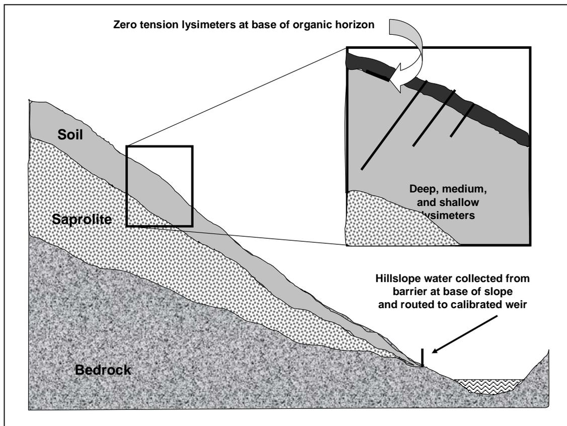
**Figure 2.2: Diagram of hillslope soil water collection. Zero tension lysimeters at the base of organic horizon, tension lysimeters at three depths within the soil. Impermeable barrier at base of slope collects all water draining hillslope into a calibrated weir, from which sample is collected.**
