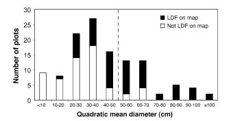
**Figure 2.** Comparison between mapped 1972 LDF condition and reference data. Inventory plots from the period (1968–1974) were geo-registered to the map and plotted here according to their measured QMD and class label. The vertical dashed line indicates the threshold used here (50.8 cm) to define LDF. Although most actual LDF was correctly mapped, some larger non-LDF was mislabeled as LDF.
