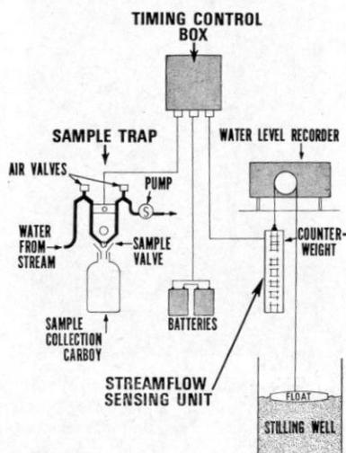
Fig. 1. Components of the proportional stream water sampler.
