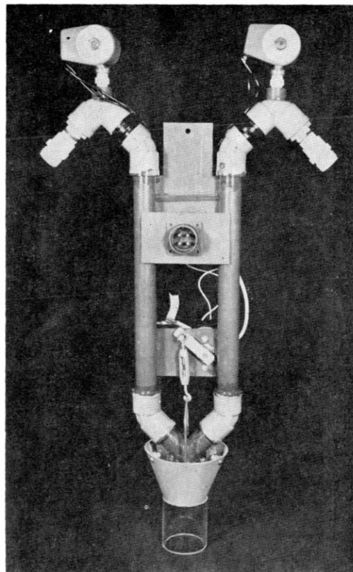
Fig. 3. The sample trap is equipped with air valves mounted on the top. A rotary solenoid operates the drain valve. The funnel fits a wide-mouth polyethylene carboy. Plumbing system from the stream attaches to the nylon hose connections. The trap is constructed of PVC pipe and fittings.
