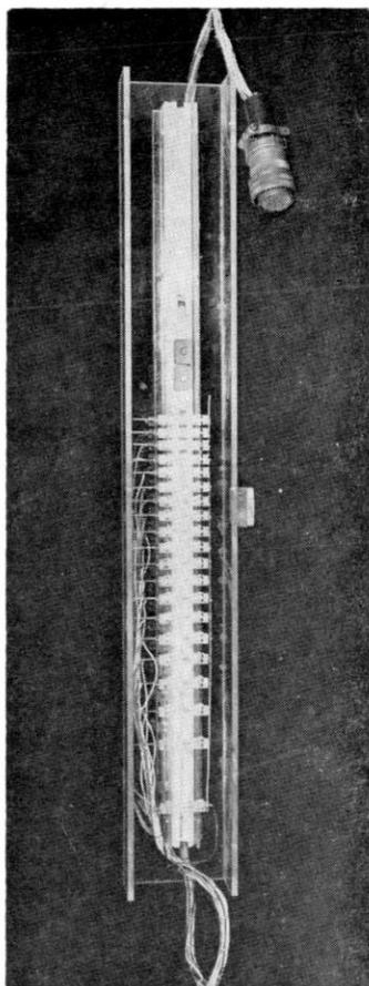
Fig. 2. The streamflow sensing unit divides the expected range of streamflows into 20 classes of equal volume flow. The counterweight on the water level recorder slides in a teflon guide. Magnetic switches are opened and closed by magnets on the counterweight with a change in streamflow.
