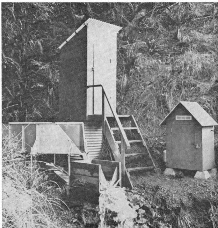
Fig. 4. A proportional water sampler samples streamflow from a 20-acre control watershed, part of a nutrient loss experiment. The study is located on the H. J. Andrews Experimental Forest 50 miles east of Eugene, Oregon.
