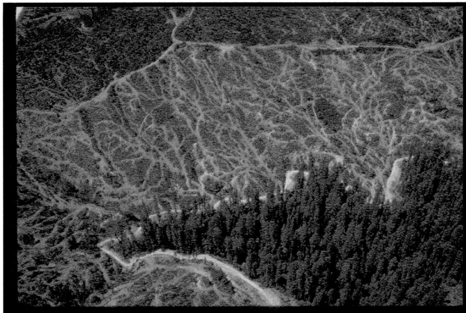
Figure 1.3b: Hillslopes in the Redwood Creek basin have a high density of skid roads and haul roads constructed during past timber harvest activities.
